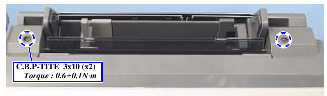
Figure 4-9. Removing the Scanner Unit
