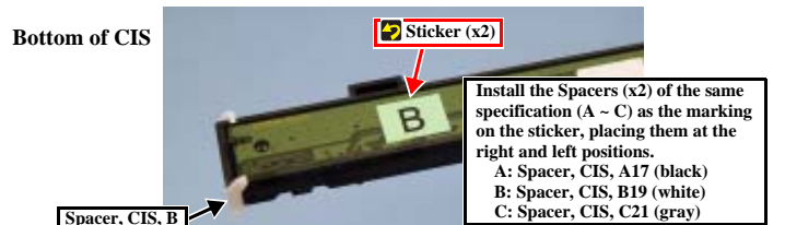
Figure 4-50. Installing Spacers CIS
