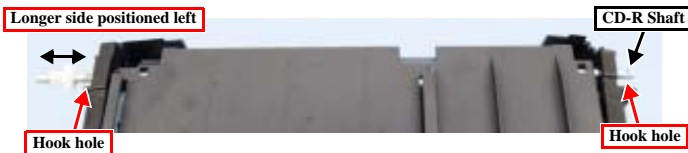
Figure 4-44. Installing the CD-R Shaft
