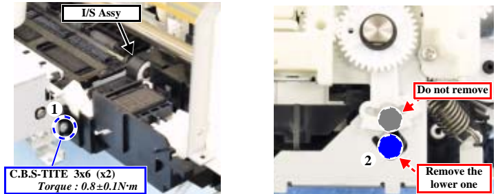
Figure 4-57. Removing the I/S Assy
