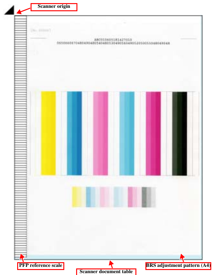
Figure 5-8. Positioning the Reference Scale and BRS Adjustment Pattern (View from Back of Document Table Glass)
