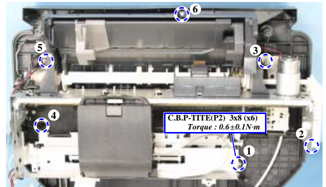
Figure 4-35. Removing the screws (Printer Mechanism Assy)
