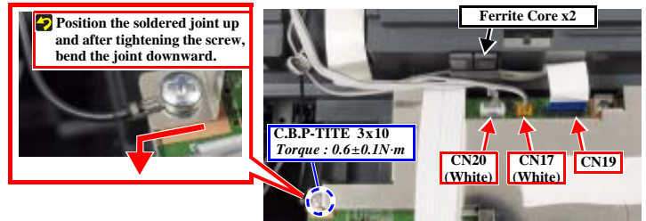
Figure 4-8. Disconnecting the cables (Scanner Unit)
