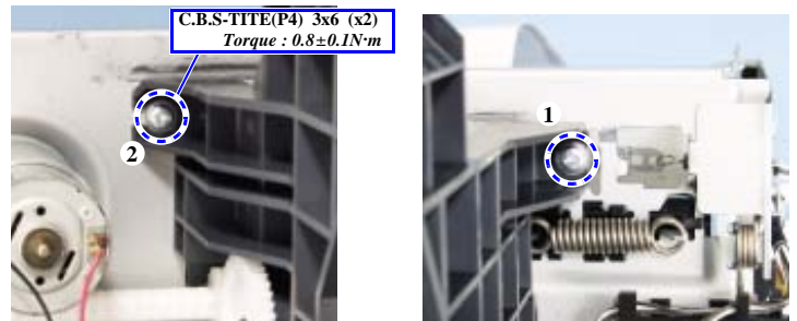
Figure 4-62. Removing the screw (ASF Assy)
