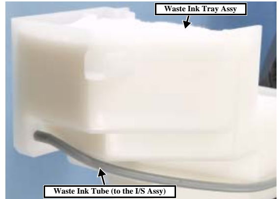
Figure 4-28. Removing the Waste Ink Tray Assy
