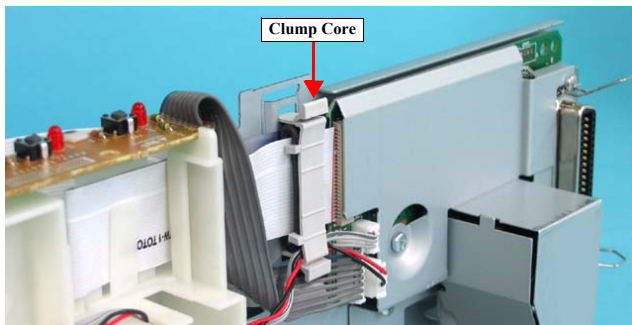
Figure 4-34. Removing Clump Core
