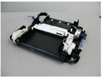
When the paper separation slope is removed as well as the printer unit from the bottom case, ink absorbers can be replaced. Some of the ink absorbers are under the paper separation slope.
