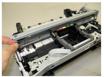
4) Remove 3 screws that fix the carriage rail to the main chassis. Before removing the center screw, remove the carriage cable holder from the front chassis. After the 3 screws are removed, slowly put down the carriage rail.
