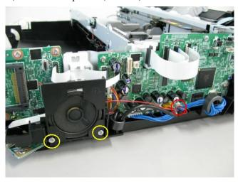
5) Remove the printer unit. (6 screws)
