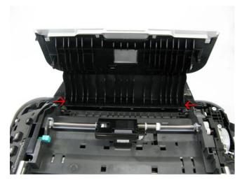
3) Remove the operation panel, eject tray, document feed switch, and document feed unit. (19 screws) <The core fits to the document feed base rib.>
