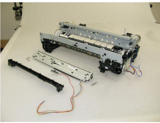
3) Remove the front chassis (3 screws).
