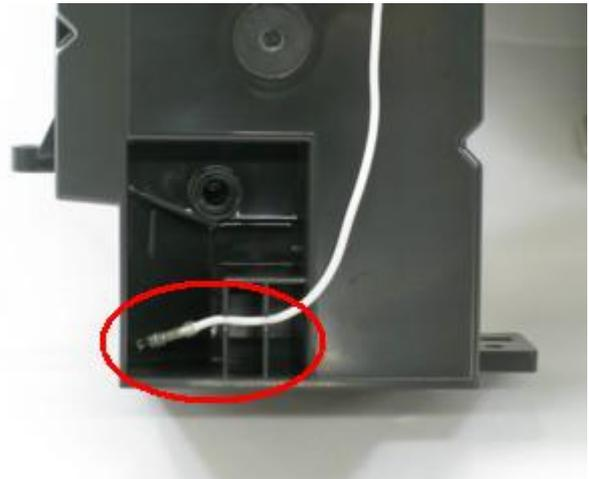
2) The ground wiring to the modular board differs between the Japan model and the other models.
