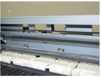
2) Remove the timing slit film. Be cautious to keep it free from any grease or damage.
