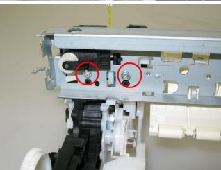
4) Separate the main chassis from the switch system unit and the purge drive system unit.
