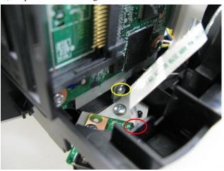
2) Separate the main PCB chassis from the bottom case. (1 screw)
