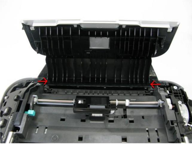
3) Remove the operation panel, eject tray, document feed switch, and document feed unit. (19 screws)
