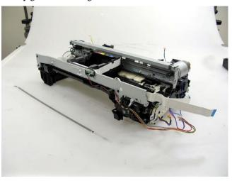
3) Using a pair of pliers, etc., release the left end of the pulley holder spring, then remove the carriage belt. Be cautious to keep it free from any grease.
