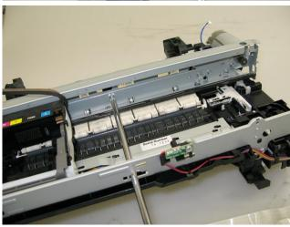
5) Remove the carriage unit. Be cautious that the grease will not attach to any parts.
