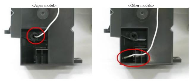
2) The ground wiring to the modular board differs between the Japan model and the other models.
