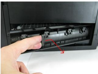
2) Remove the AC adapter. (1 screw) <Pull out the AC adapter from the bottom of the bottom case.>
