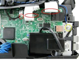
5) Remove the side cover L, disengage the scanner support, then separate the scanner from the printer. (4 screws)
