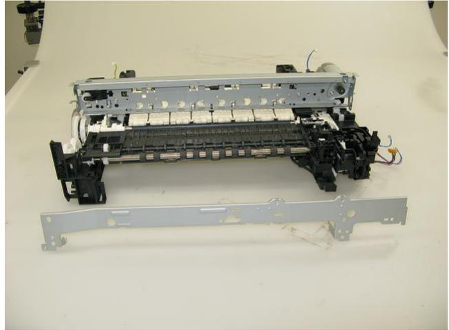
4) Unlock the paper eject roller gear. While raising the front of the platen unit, remove the platen unit from the printer unit.
