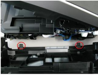
4) Remove the scanner cable, LCD cable, document feeder harness, panel ground harness, and core. (1 screw) <The core fits to the main case rib.>
