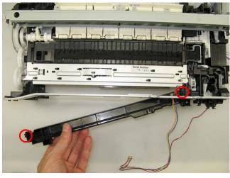
2) From the left and right sides of the spur unit, release the springs (2 on the left side, 1 on the right side). Then, slowly pull the spur unit upward to remove it from the platen unit.
