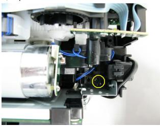
3) Separate the PCI DC and GND harnesses from the printer unit. (1 screw) <The GND harness fits to the bottom case rib.>
