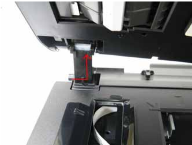
6) Separate the scanner from the document feeder. (no screws)
