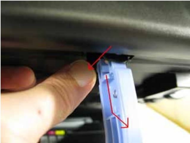
6) Separate the scanner from the document feeder. (no screws)
